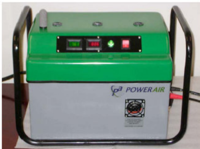
Caption: PWAC Portable Emergency Generator (Prototype)
