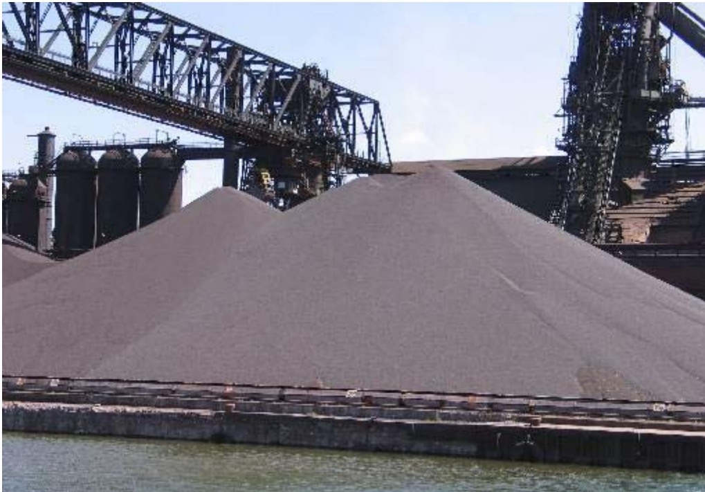
This heap of iron ore pellets will be used in steel production.
